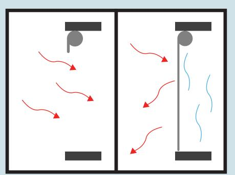
Utilization of shades to regulate building temperature
